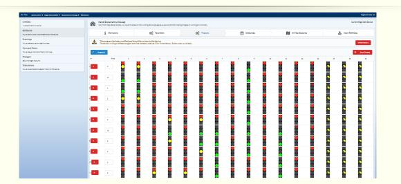
TEST PROCEDURE: The cards and the groups defined on the device used with the service purpose are displayed on the screen as a representative of the traffic lights by clicking on the mouse with the individual desired lamps flashing mode. Thus, it is much easier to detect line faults and correct faults are eliminated in a short time.
